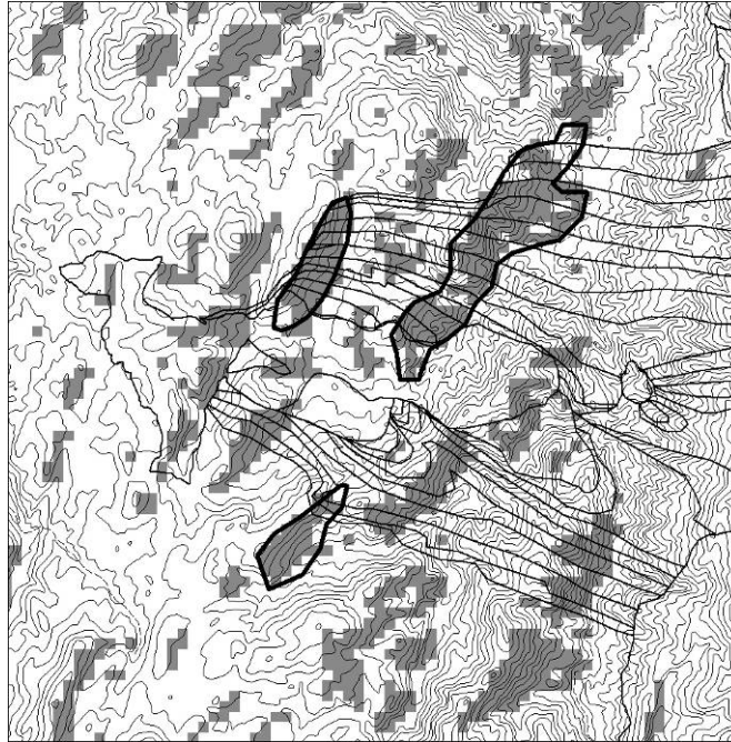
Figure 6. Example of output from the model (equation (1)) for identifying channelling prone parts of the landscape (indicated in grey). Thin black lines are 10-minute isochrones of the Broken Cart Fire derived from the line-scan data, showing the influence of three events (outlined) on lateral spread. The model was applied assuming \theta_w = 112.5^\circ and parameter values of \sigma = 10.5^\circ and \delta = 33^\circ .
