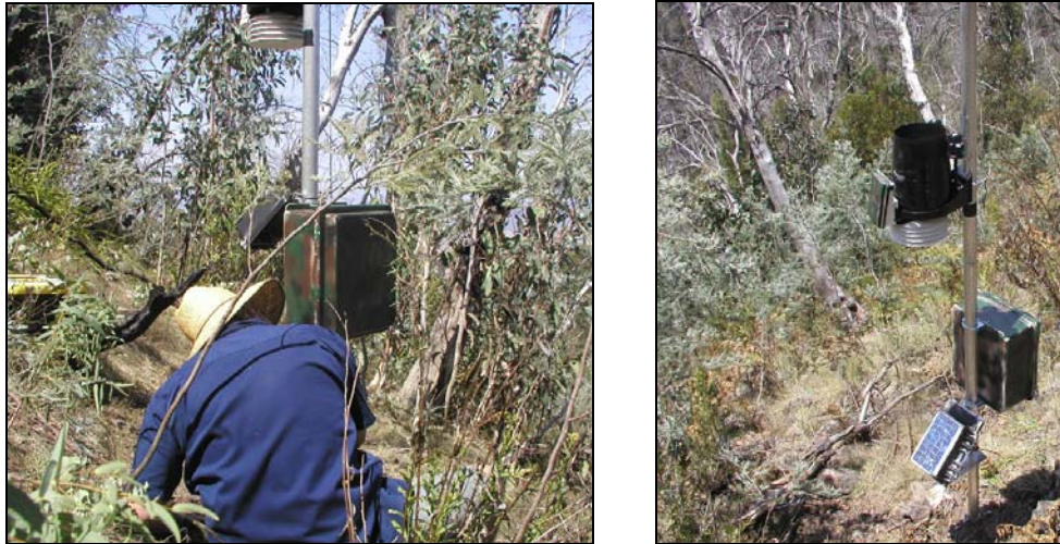
Figure 1. Installation of a portable automatic weather station on a very steep, fire-affected slope of the Tidbinbilla Range. This is one of a dozen stations, that carry sensors for a wide range of weather parameters, and which require no site disturbance to install.
