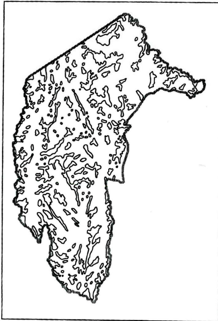
Figure 4. Zero meso-scale elevation residual contours, as produced by the detrending model (reduced from original scale, with some subsequent loss of detail).
